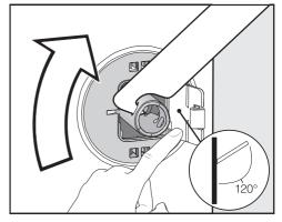
■ Push the flap outwards and turn the transit bar 90° using the enclosed spanner.
