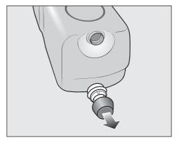
Remove the cover caps from the detergent cartridges included with the delivery.
