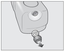
Remove the cover cap from the cartridge.
