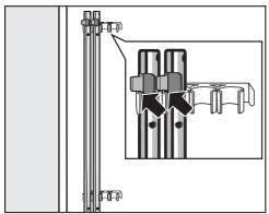
Secure the transit bars to the back of the washing machine. Make sure that the top catch is located above the holder. Nisk of damage from incorrect transport.
