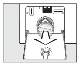
■ Remove the drain filter completely.
