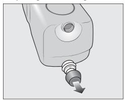
Remove the cover cap from the cartridge.
