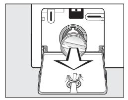
■ Remove the drain filter completely.
