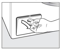
■ Open the drain pump access panel.
