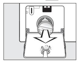
■ Remove the drain filter completely.
