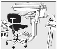
Ensure that the ironer is level so that steam is emitted evenly. Ensure that the ironer is sufficiently stable to prevent it from rolling sideways.
