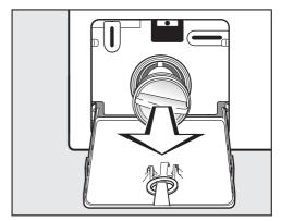
■ Remove the drain filter completely.
