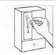
■ Switch the flatwork ironer on by pressing the "On / Off" () button.
