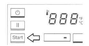
The "Start" button begins to flash as soon as the flatwork ironer has reached the minimum temperature.
