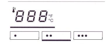
■ Set the corresponding heater plate temperature according to the type of fabric.
