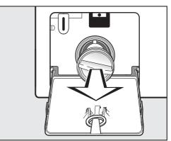
Remove the drain filter completely.
