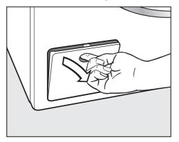
Open the access panel for the drain pump.
