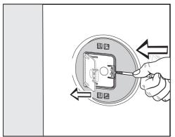
Press against the retainer with a sharp object (a narrow screwdriver, for example).
