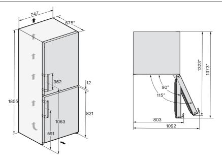
$^{\ast}$  Dimensions without wall spacers fitted. Appliance depth is increased by 15 mm with the wall spacers supplied fitted.
