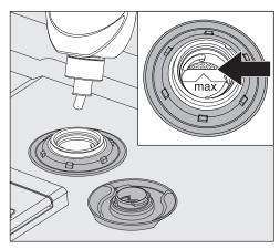
■ Add the process chemical only until it is visible at the "max" mark in the funnel.
