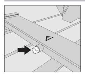
■ To measure the wash pressure, replace the blind stopper with a Luer Lock adapter.
