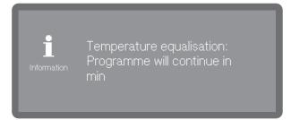
If the temperature inside the wash cabinet is more than 60 °C at this point, the pressure is equalised first. Then the programme continues.
