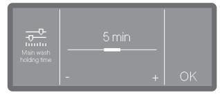
Set the holding time and press OK to save the setting.
