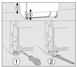
The front machine feet can be adjusted with an open spanner (spanner size 13); the rear ones with a T20 Torx screw.
