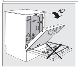
■ Open the door to an angle of around 45°. This ensures that the salt flows into the container more easily.
