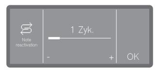
Cancelling machine lock due to lack of salt If the salt in the water softener has been used up, a fault appears on the display and the machine is locked to prevent further use.
