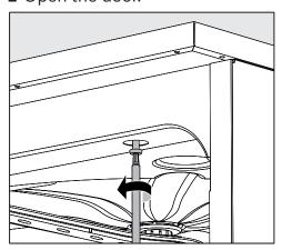
■ Remove the cover caps on the left and right and tighten the fixing screws. Then refit the cover caps.
