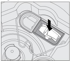
The drain pump impeller is situated under the non-return valve.
