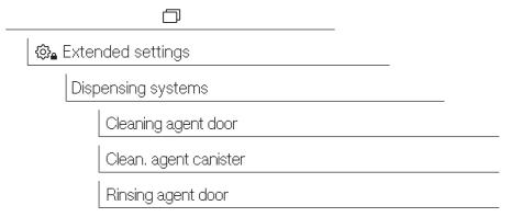
Only the available dispensing systems are displayed. Activated dispensing systems are highlighted by a  $\bigcirc$  tick. Deactivated dispensing systems are preceded by a  $\bigcirc$  circle symbol.
