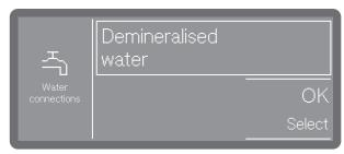
The frame indicates the activated water connection. Tapping the connection removes the frame and permanently deactivates the water connection.
