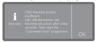
■ Follow the instructions on the display and top up the reactivation salt, see (i) "Filling the container for reactivation salt".
