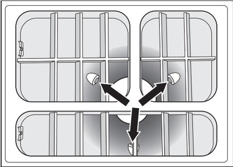
A technical diagram of the coffee bean container. It shows two bean containers on top and a larger container below. Three arrows point to small circular sensors located on the top surface of each of the two upper containers and on the top surface of the lower container.</div> <ul style="list-style-type: none"><li>■ Rengjør oppfyllingssensoren (se bilde) med en myk, tørr klut.</li></ul> |
