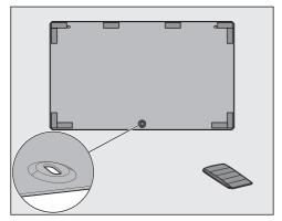
■ Stick the sealing strips from the accessory pack to the inside of the rear panel as shown in the image.
