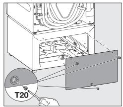
■ Use the raised head screws to screw the prepared panel to the rear of the base.
