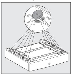
■ Stick the sealing rings to the underside of the stacking kit.
