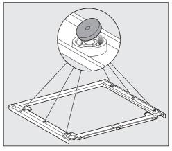
■ Stick the 6 sealing rings to the underside of the stacking kit.
