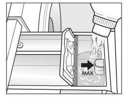
■ Add the fabric softener or the liquid starch to the ⊗ compartment. **Do not exceed the maximum level mark.**
