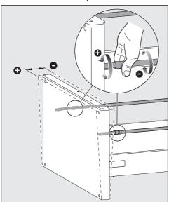
■ To adjust the inclination of the drawer, turn the two rails.
