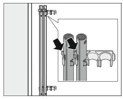
Secure the shipping struts to the rear panel of the washing machine. Make sure that the top retainer is located above the holder.
