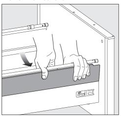
■ Push the top panels outward from inside and set the panels aside.
