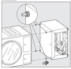
Place the spacer sleeves on the set screws. Push the base and the washing machine together. The set screws must be inserted in the holes of the feet that have been removed from the washing machine.
