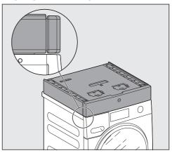
Align the stacking kit centrally and make sure it is flush with the front of the washing machine.
