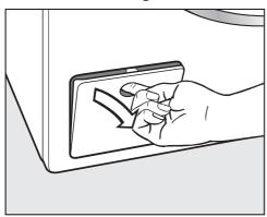
■ Open the drain pump flap.
