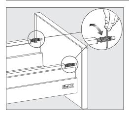
■ To adjust the inclination of the drawer, turn the two rails using a screwdriver.
