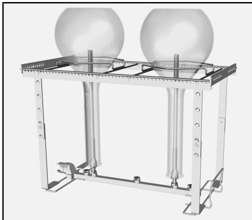
The measuring flasks rest on the support in the module frame. The cone on the bottom of the injector nozzle should be inside the neck of the item. This protects the rim from becoming chipped.
