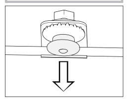
Carefully pull down the pressure cap. The browning/broiling element then lowers automatically.
