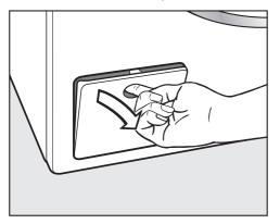
Open the drain pump access panel.
