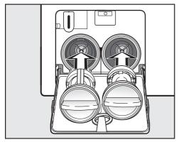
Replace the filters correctly (on the right and left) and tighten them.
