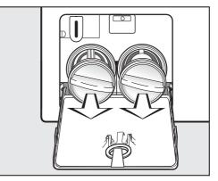
Remove the filters completely.
