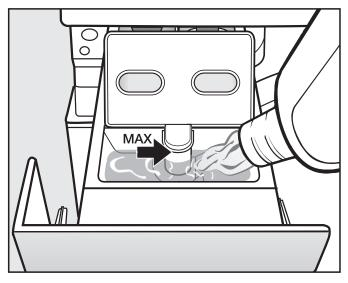
Add the fabric conditioner or liquid starch to compartment <sup>(8)</sup>. Do not exceed the maximum level mark.
