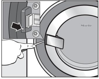
4 mm blade) into the opening next to the door lock and use it to release the catch. Turning it slightly in an anticlockwise direction should release the door.
