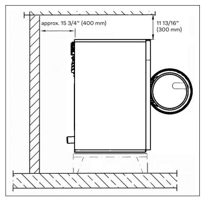
Minimum safety distance to the wall approx. 15 3/4" (400 mm) to allow for maintenance.
