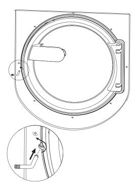
■ Using a T 40 Torx wrench, turn the release element with the inner hexagon 2 whole revolutions in the direction of the arrow.
