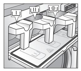
■ For standard wash programs, add powder detergent for the main wash to the Ш compartment and if desired, add detergent for a pre-wash to the U compartment. Add fabric softener to the front of the 🖹 compartment.
