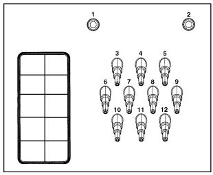
Connections **1** and **2** are provided for viscous agents. These connectors are closed and must be drilled open using an 8 mm bit.
