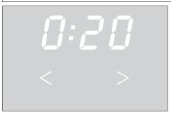
■ Touch the < or > sensor button repeatedly until the required program runtime appears on the time display.
