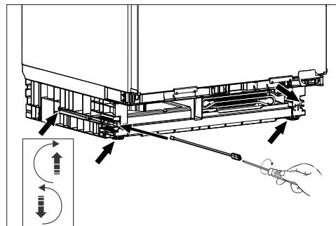
■ Adjust both rear feet with appropriate screws at the front right and left in the base using the rod supplied and a flat-head screwdriver.
