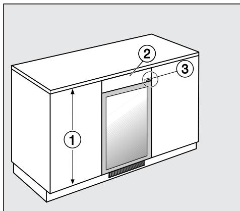
If adjacent cabinet fronts (1) are taller than the wine refrigerator door, the wine refrigerator can be aligned with the adjacent cabinet fronts using a filler panel (2).
