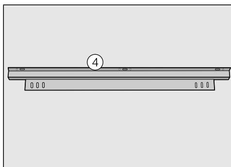
A fixing bracket (4) is required to secure the filler panel. This is available from Miele Service or from specialty dealers. The fixing bracket is installed on the wine refrigerator:
