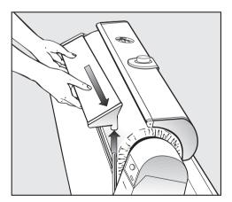
■ Remove the feed-in table as described in the section "Ironing".
