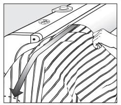
Pull the shirt over the roller as far as the yoke seam - or to the collar seam on shirts without a yoke - and smooth it out.
