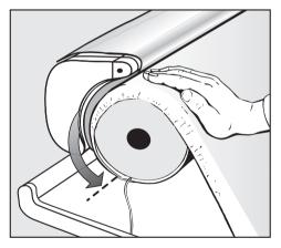
■ Turn the roller by hand in the direction you iron (see arrow) until the cover retaining slot is at the bottom.
