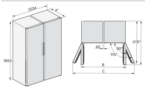
$^{\ast}$  Dimensions without wall spacers fitted. Fitting the wall spacers supplied increases the appliance depth by 15 mm.
