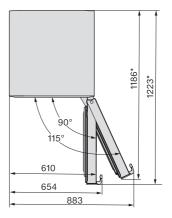
\* Dimensions without wall spacers fitted. Appliance depth is increased by 15 mm with the supplied wall spacers fitted.
