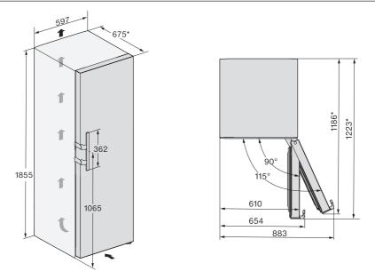
\* Dimensions without wall spacers fitted. Fitting the wall spacers supplied increases the appliance depth by 15 mm.
