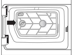
3 Press the frame of the filter insert in at the positions marked PUSH until it audibly engages.
