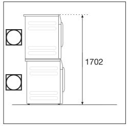
2 Miele tumble dryers can be installed as a dryer stack. A stacking kit\* is needed for this purpose. This must be fitted by a Miele authorised technician.
