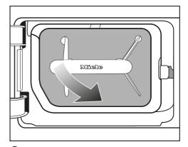
Use the handle to pull out the plinth filter forwards <u>at an angle</u> and to the right.
