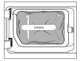
The edges of the filter do not sit properly and the filter is deformed. Fluff will blow into the heat exchanger unfiltered through edges that do not sit properly. This will cause a permanent obstruction in the heat exchanger.
