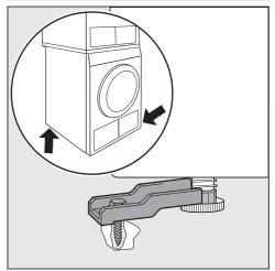
■ Secure 2 feet to the tumble dryer diagonally at the front and rear or only at the rear.
