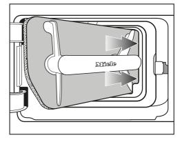
Use the handle to slide the fluff filter on the right <u>at an angle</u> behind the edge.
