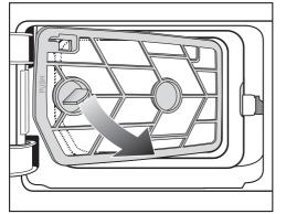
Use the handle to pull out the filter insert <u>at an angle</u> forwards and to the right.
