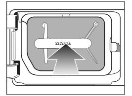
2 Then press on the handle until the fluff filter is secured in position.
