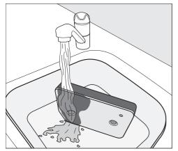
**Tip:** To speed up the removal of residue from the surface, run a water jet vertically over the front of the plinth filter.
