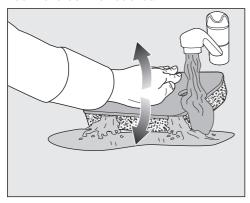
To efficiently loosen underlying residue, gently press down on the plinth filter with the back of your hand.
