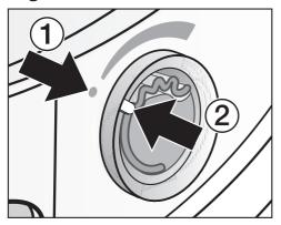
■ Turn the outer ring anti-clockwise until the markers ① and ② line up.
