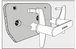
■ Pull the handle out of the plinth filter.
