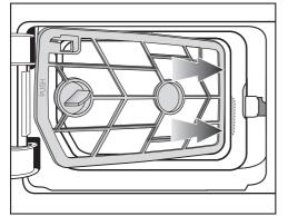
① Use the handle to slide the filter insert to the right at an angle behind the edge.
