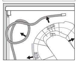
■ Pull the drain hose out of the clips.
