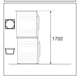
A stacking kit\* (APCL 001) is required. This must be fitted by a Miele authorised technician. Secure the washing machine using the fastening bracket supplied with the machine.
