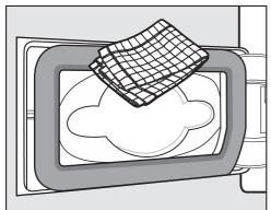
Use a damp cloth to remove any fluff. Make sure that you do not damage the rubber seal when doing this.
