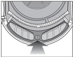
■ Push the lower fluff filter in completely and lock it with the yellow rotary control.
