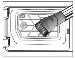
Carefully vacuum up any visible fluff or soiling. Use a dusting brush or the narrow crevice nozzle.
