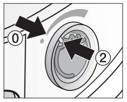
■ Turn the outer ring anti-clockwise until the marker ② is in position ③.
