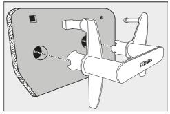
■ Fit the fluff filter back on the handle. Make sure it is the correct way round.
