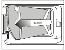
2 Pull the plinth filter out at an angle.
