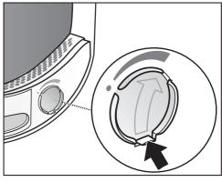
Open the cover using the tab until the tab is right at the top.
