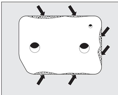
**!** Damage caused by a damaged or worn plinth filter.
