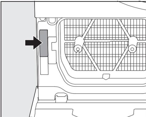
A fastening element (arrow) is activated when the holder is pulled out. The fastening element prevents the plinth flap from closing without the holder inserted. The fastening element is deactivated when the holder is pushed in.
