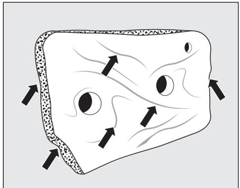
Deformations can be seen on the side edges and on the entire plinth filter.
