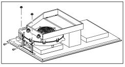
Undo the fixing brackets.
