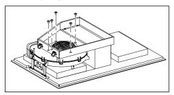
Undo the 5 screws on the fan.
