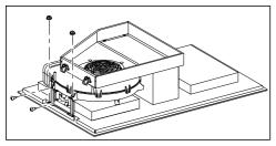
Undo the fixing brackets.
