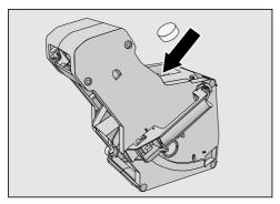
Drop a cleaning tablet into the top of the brew unit (arrow).  Push the brew unit containing the cleaning tablet back into the coffee machine.
