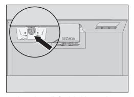
Clean the milk flask holder on the coffee machine with a damp cloth.
