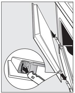
Hold the door securely on both sides and carefully fit it back into the hinge retainers.
