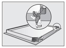
Flip both the glass pane retainers inwards in such a way that they fit over the lower of the two middle panes. Refit the upper of the two middle panes in such a way that the material number is legible (i.e. not reversed). The pane must rest on the retainers.
