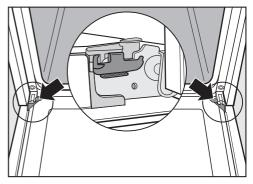
The oven door is connected to the door hinges by retainers.
