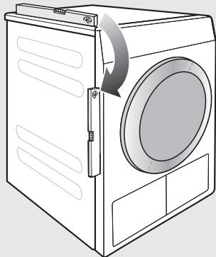
The appliance must stand perfectly level on all four feet to ensure safe and proper operation.
