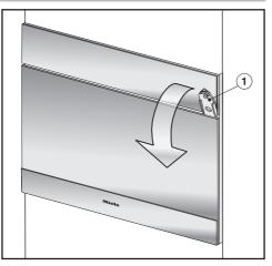
Insert the opener included with the appliance ① about 3 cm into the gap between the door and the control panel on the right-hand side and then pull the door open. Risk of injury caused by hot surfaces and food.
