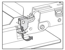
Release the locking clamps on the hinges by turning them upwards as far as they will go until they are at an angle.
