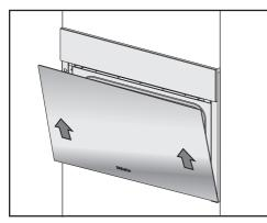
Hold the door securely at both sides and lift it evenly upwards off the hinge retainers.
