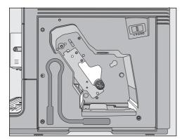
Clean the interior of the coffee machine. Make sure that the areas highlighted in the illustration are cleaned especially well.
