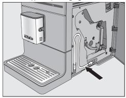
The milk pipework is located behind the appliance door.
