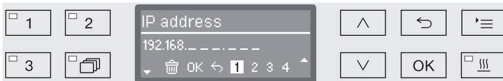
The current setting is shown on the middle line of the display. It can be changed using the options shown in the bottom line. The top line shows which option has been selected from the bottom line. The following data entry options are available:
