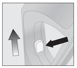
Press the release button and remove the Comfort handle by pulling it upwards.
