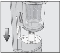
■ Slide the dust container handle along the guide line and down onto the PowerUnit connector from above until the dust container audibly clicks into place.
