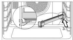
■ Slide the FlexiClip runner at an angle along the top rail as far as it will go (3.).
