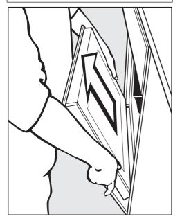
Hold the door on either side and pull it diagonally upwards off the retainers. Make sure that the door is straight.
