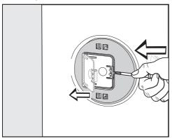
■ Press against the retainer with a sharp object (a narrow screwdriver, for example).
