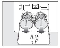
■ Remove the drain filters completely.
