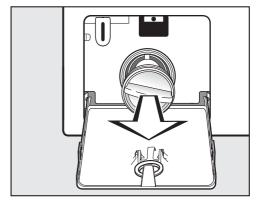
■ Remove the drain filter completely.
