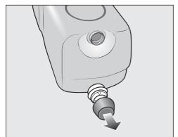
Remove the cover cap from the UltraPhase 2 detergent cartridge included with the delivery.
