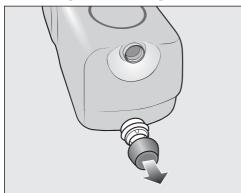
Remove the cover cap from the cartridge.
