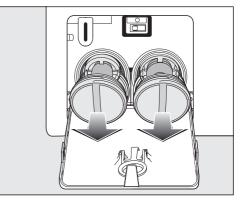
■ Remove the drain filters completely.
