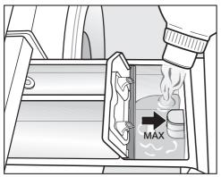
Add fabric conditioner or liquid starch to the & compartment. Do not exceed the maximum level mark.
