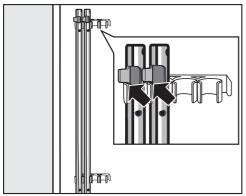
Secure the transit bars to the back of the washing machine. Make sure that the top catch is located above the holder. Risk of damage from incorrect transport.
