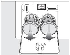
■ Remove the drain filters completely.
