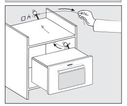
■ Slide the appliance into the niche. Feed the cable with the plug through the back of the furniture unit.
