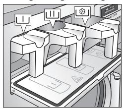
■ For standard wash programmes add the powder detergent for the main wash to the Ш drawer and if desired, add detergent for a prewash to the Ш drawer. Add fabric conditioner to the front of the drawer.
