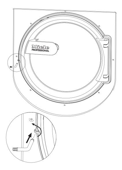
■ Using a T 40 Torx wrench, turn the release element with the inner hexagon two whole revolutions **anti-clockwise** (left).
