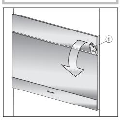
■ Insert the opener ① supplied about 11/2" (3 cm) into the gap between the door and the control panel on the right-hand side and then pull the door open.
