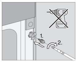
Insert the bolt into the mounting aid and tighten it in the housing unit. Do not use a cordless screwdriver.
