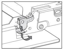
Release the locking clamps on the hinges by pushing them down as far as they will go until they are at an angle.
