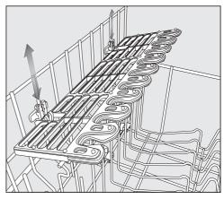
■ Slide the glass rack to the desired height until the catches click into place at the top or the bottom.
