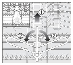
■ If the bottle holder is not needed, lift it up using the yellow lever ① and fold it to the side ②.
