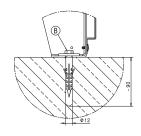
Dimensions in mm B Screw/anchor point
