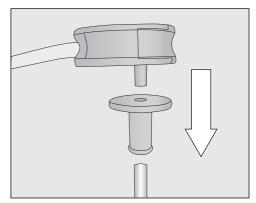
First insert the connecting piece onto the long stainless steel tube (milk siphon). Make sure that the slanted end of the stainless steel tube is pointing downwards.
