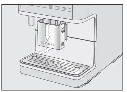
Slide the central spout right down and remove the stainless steel cover by pulling it off towards you.
