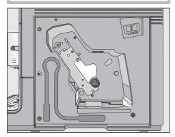
Clean the interior of the coffee machine. Make sure that the areas highlighted (in white) in the illustration are cleaned especially well. **Useful tip:** Use your vacuum cleaner to remove dry ground coffee residues.
