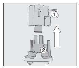
Remove the upper silicone piece with the holder for the milk pipework ①.
