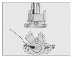
Bend the cleaning brush slightly and clean both spouts from the top and bottom.
