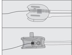
Also clean the hose connections in the rinsing valve body: to do this, insert the cleaning brush in each opening and move the brush back and forth.
