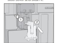
■ Detach the milk pipework from the dispensing unit 1. Pull the dispensing unit down to remove it 2.
