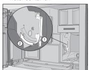
■ Press the button under the handle of the brew unit 1 and, while doing so, turn the handle forward (2).
