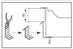
Secure the hob using the brackets supplied.
