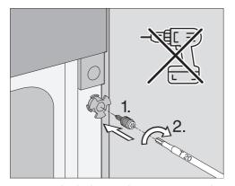
■ Insert the bolt into the mounting aid and tighten it in the housing unit. **Do not** use a cordless screwdriver.
