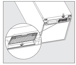
Place the rear edge of the insect protection panel in the rear groove of the recess.
