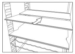
■ Lift up the front section of the glass shelf slightly at the front and slide it carefully underneath the rear section.
