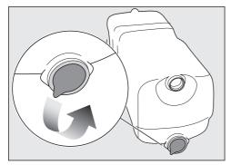
■ Remove the film seal from the cartridge completely.
