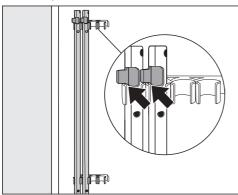
Secure the transit bars to the rear panel of the washing machine. Make sure that the top retainer is located above the holder.
