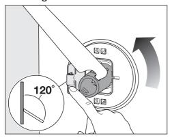
■ Push the safety cap cover out by 120° and turn the transit bar 90° using the open spanner supplied.
