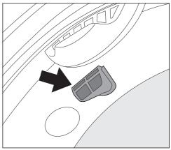
■ Remove the fluff with your finger. Do not use any sharp or pointed tools to do this.
