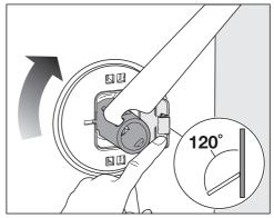
■ Push the safety cap cover out by 120° and turn the transit bar 90° using the open spanner supplied.
