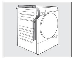
■ Use a spirit level to check the washing machine is standing level.
