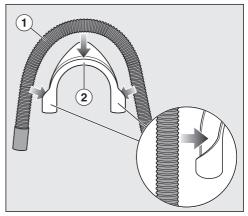
■ Insert the drain hose ① into the swivel elbow ②.
