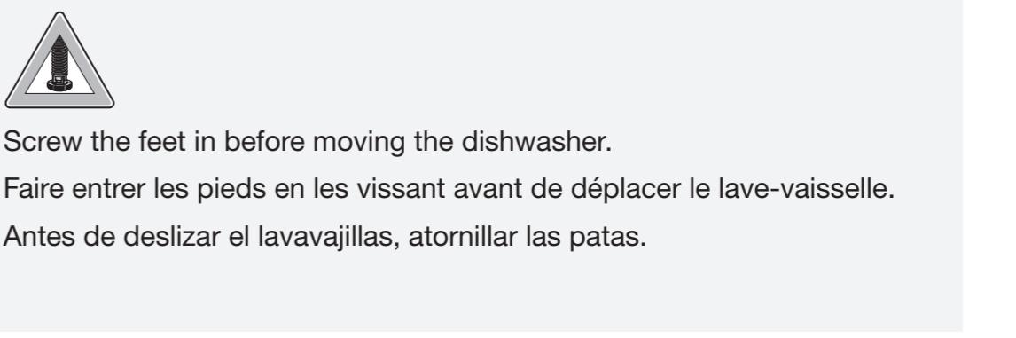
Screw the feet in before moving the dishwasher.
