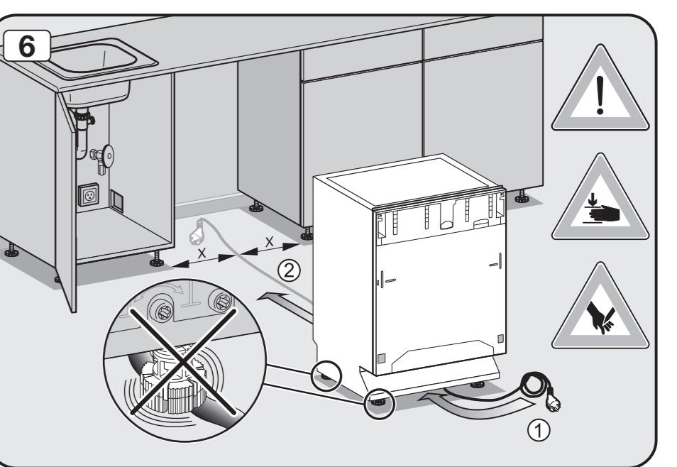
If the intake hose will be coiled under the dishwasher after it is inserted in its niche, the undercounter height must be at least 32 7/16" (835 mm) for standard height models or 34 13/16" (885 mm) for XXL height models. **Do not** sit the dishwasher on the hose. The hose needs to be free of kinks and able to move freely after installation. **Do not** place hose or power cord next to a heat source e.g. hot water pipes. **Do not** expose hose or power cord to corrosive substances.
