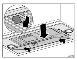
To take out the grease filter, release the locking clip on the filter, lower the filter approx. 45°, unhook it at the back and remove it
