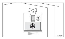
In recirculation mode the silencer needs to be positioned between the exhaust connection and the exhaust grille ②. Please ensure there is adequate installation space.
