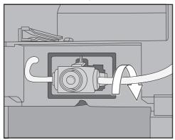
**Tip:** If necessary, screw the milk pipework backward at the connecting piece on the right-hand side.
