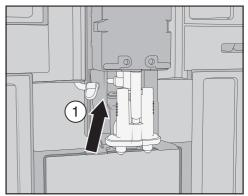
Detach the milk pipework from the dispensing unit as follows: pull the pull tab ① to the left.
